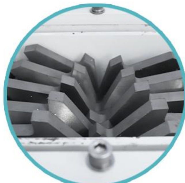
Single Shaft (For shredding glass-based medicines)
